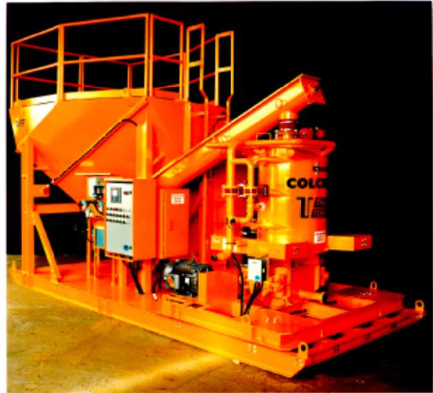
FIG 5 - The Thiessen Tornado 1000 - A PLC controlled grout slurry plant with 6.5 tonne cement hopper and 1000 litre colloidal mixer.
