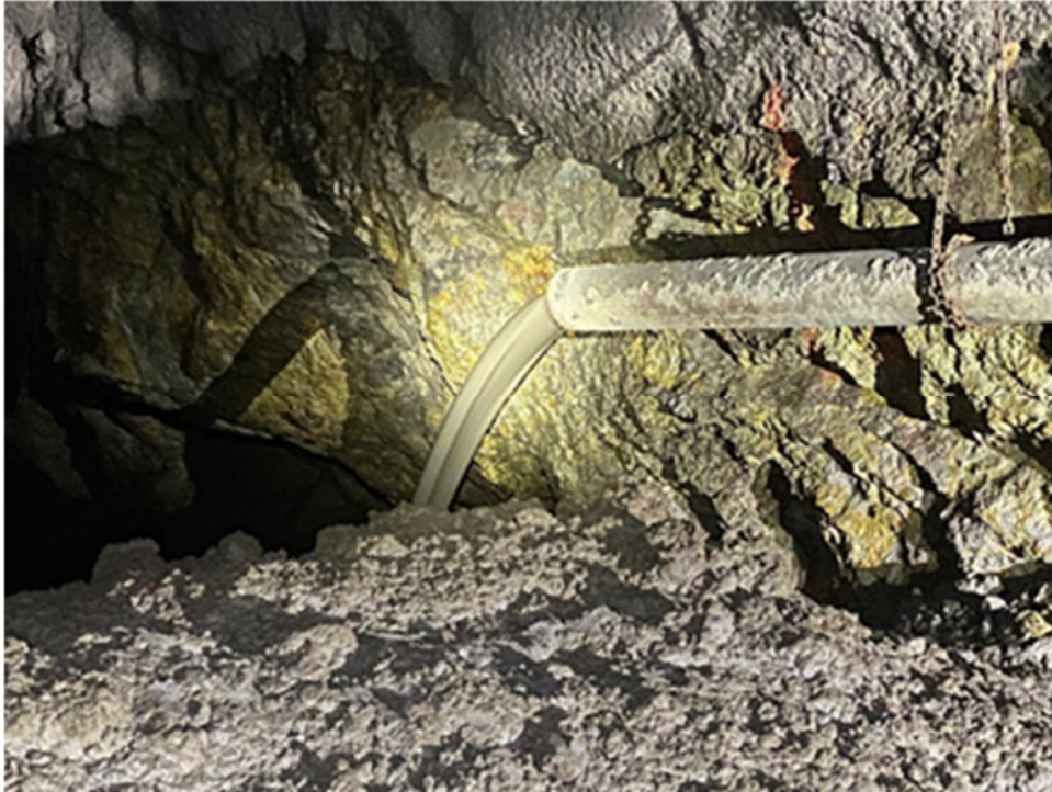
Figure 12 First cemented paste pour at FDN
