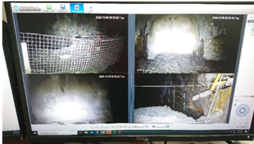
Figure 17 Live underground monitoring for paste operators
