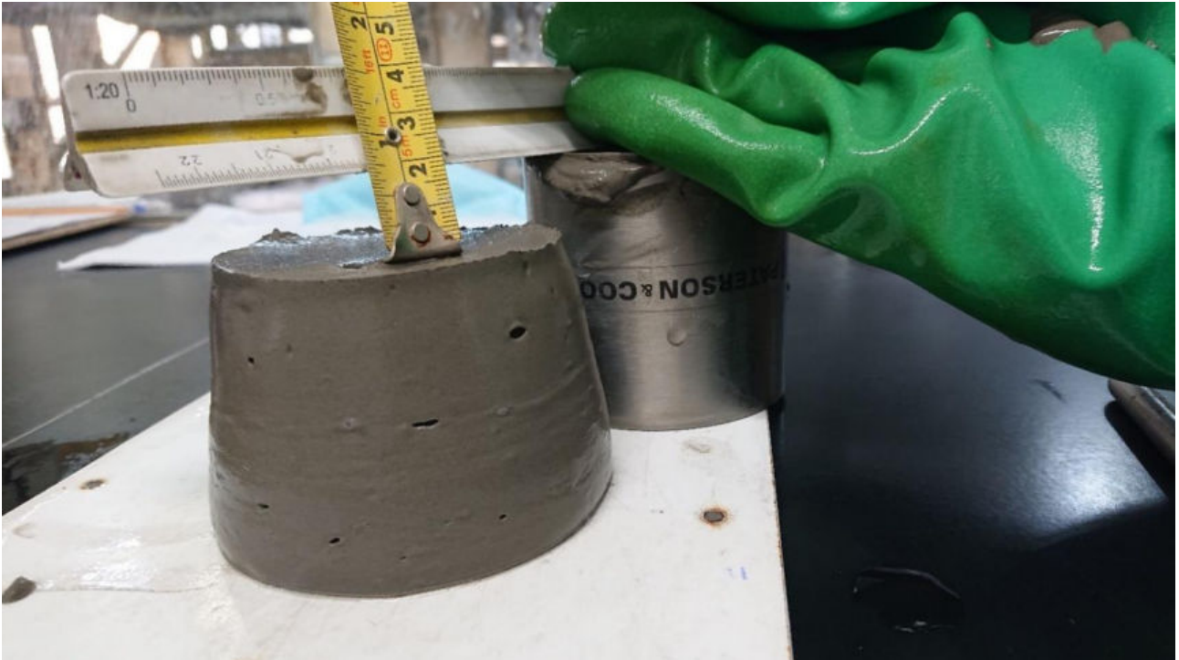
Figure 4 Paste sample leaving the mixer (deslimed tailings, 71% m )
