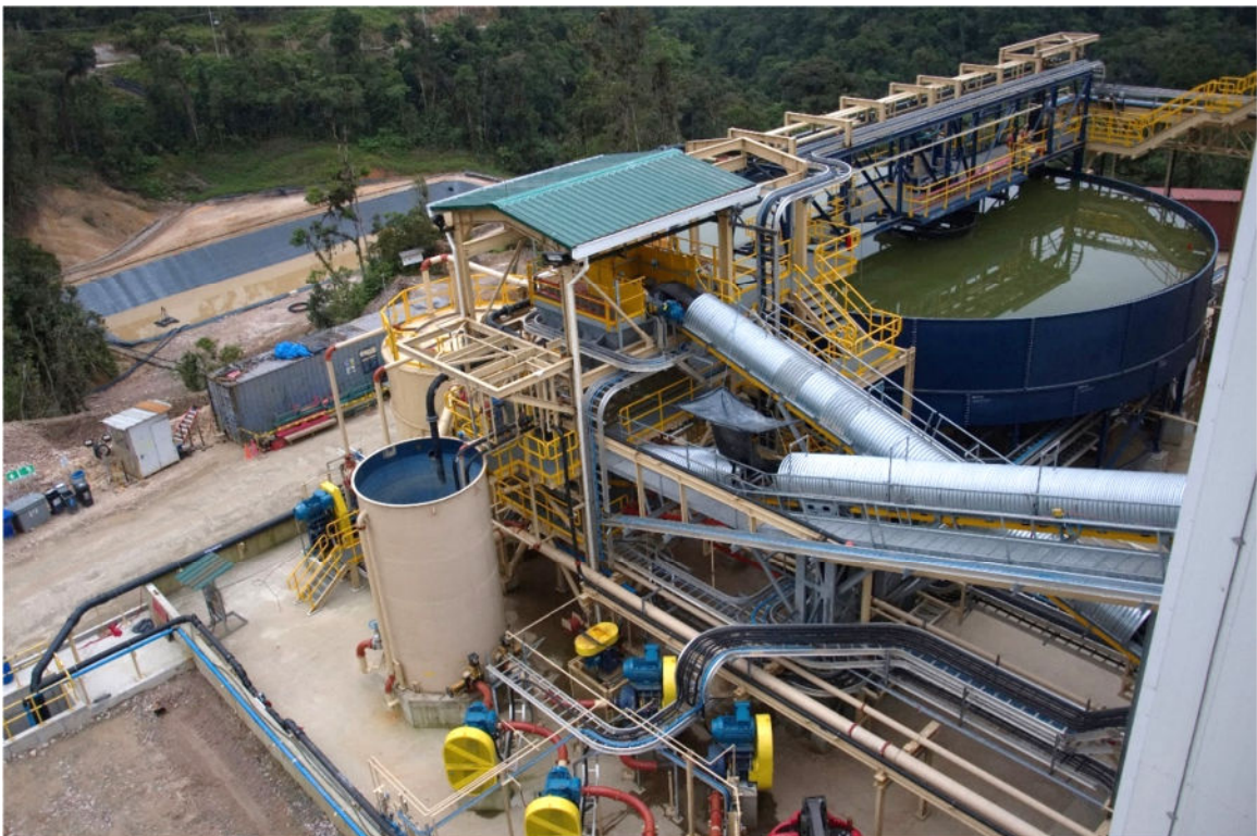
Figure 10 Tailings feeder with switchback conveyor arrangement
